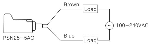
※ The load can be connected to either wire.
