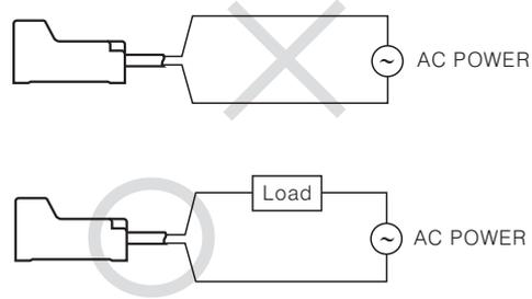
When using DC 2-wire and AC 2-wire type, a load must be connected before applying power; otherwise, components can be damaged.
