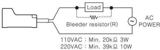
It may cause return failure of load by residual voltage.
