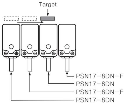
When installing several proximity sensor closely, it may cause malfunction due to mutual interference. Therefore, please use differential frequency for the application.
